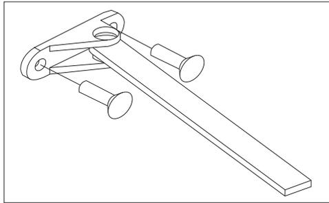
2. For pull systems, slide the pull arm roller into the track, then insert a track cap on each end of the track and attach the track to the door:
